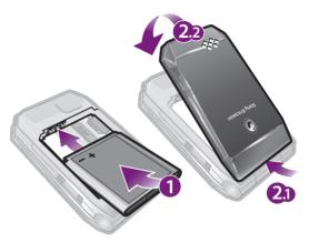
1 Insert the battery with the label side up and the connectors facing each other.
