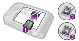
Remove the battery cover and insert the memory card with the gold-coloured contacts facing down.
